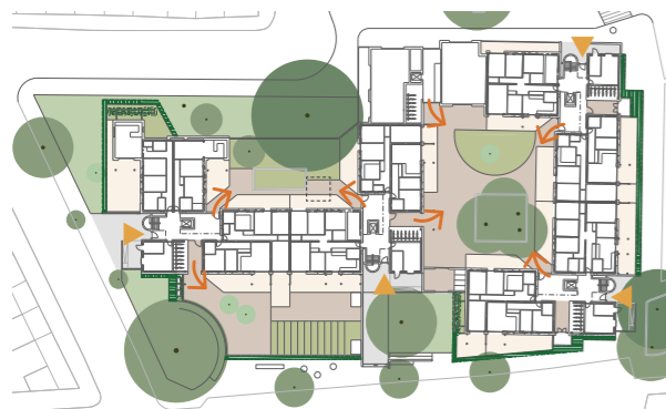
A proposed ground floor plan for Cannington and Langridge, two blocks to the south of the site, showing enclosed communal external areas
